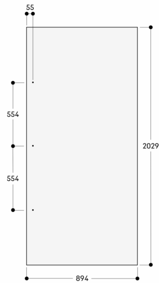
The door panel thickness is 19 mm The maximum door panel dimensions are based on a clearance of 3 mm, based on a single niche Measurements in mm
